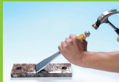
The grip end can be used as a point to contact for hammering.
