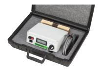
The Ammeter Shunt Kit is used to verify magnetizing current output of magnetic particle inspection equipment up to 10,000 amps on half-wave DC, 1-phase full-wave DC and 3-phase full-wave DC output, and up to 6,000 amps on AC current output.
