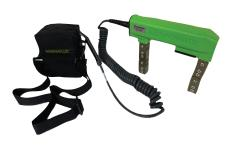
The Y-8 is a battery-powered, DC electromagnetic yoke designed to stand up to the most rugged applications. Its compact battery pack provides a full 8-hour shift of inspection power, making it ideal for inspection in the field and remote locations.
