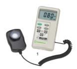
The Visible Light Meter accarately measures visible light in either foot-candles or lux and includes a permanently affixed visible light sensor specially constructed to measure visible white light in the range of 400-760 nm for non-destructive testing.
